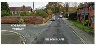
With regard to our request for centreline marking CoYC TM state that this is not used on roads with an overall width of less than 5.5m and as much of Nelsons Lane is under that limit the use of such a line would not be recommended. CoYC TM seem to have ignored the fact that we were only looking for a centre-line marking through the s-bends in the vicinity of the children's play park.
